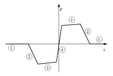
Because the ball is spherical and the notch is symmetric, the horizontal force versus displacement function is symmetric about the origin. (See "Peak Force and Notch Width" on page 1-318.)
