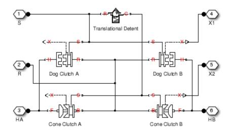
The model implements two Dog Clutch blocks, one Translational Detent, and two modified Dog Clutch blocks. Refer to each block reference page for more information on the corresponding block function.
