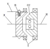
The schematic illustrates a synchronizer in the disengaged state. In this state, the ring (R) and hub (H) shafts can spin independently at different speeds. To synchronize ring
