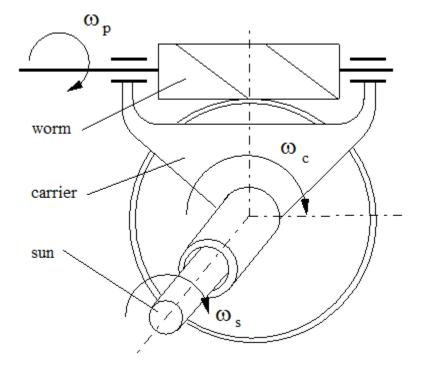
You specify a fixed gear ratio, which is determined as the ratio of the worm angular velocity to the sun gear angular velocity. You control the direction by setting the worm thread type, left-handed or right-handed. Rotation of the right-handed worm in positive direction causes the sun gear to rotate in positive direction too. The positive directions of the sun gear and the carrier are the same.
