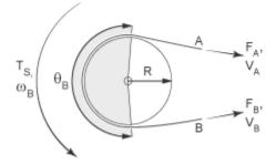
For a flat band, specify the value of f directly in the block parameters dialog box. For a V-belt, the model calculates the value using this equation:
