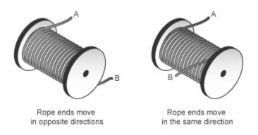
During normal operation, a driving torque causes the cylindrical drum to rotate about its symmetry axis. The rotating drum transmits a tensile force to the rope ends, which translate with respect to the drum center line. The relative direction of translation between the two rope ends depends on the rope windup type. However, a positive drum rotation always corresponds to a positive translation at rope end A.
