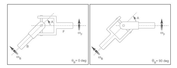
In the figure, the intersection angle is the angle between the two shafts about the base shaft's pin. The absolute value of this angle must fall in the range O#A<Maximum intersection angle. The base shaft angle is the angle of the base shaft about its length axis. The base shaft angle is also the time-integral of the base shaft angular velocity,  $\omega_B$ .
