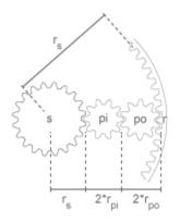
In terms of the ring-sun and outer planet-inner planet teeth ratios, the ring-outer planet teeth ratio is
