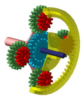
The stepped planet gear set enables a larger speed-reduction ratio in a more compact geometry than an ordinary planetary gear can provide. The compound reduction ratio depends on two elementary reduction ratios, those of the sun-large planet and ring-little planet gear pairs. Because of this dependence, compound planetary gears are also known as dual-ratio planetary gears. For more information, see "Compound Planetary Gear Model" on page 1-34.
